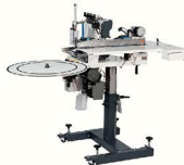
V700 Automatic pocket hemming unit 2CS
