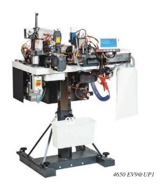
tory. The wiper has been replaced with a new top efficiency thread blowing device. This means more efficiency and no more parts to replace.
