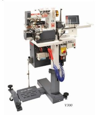
The latest direct drive motor and the refined puller applied to this unit allow increased efficiency, improved sewing and cutting performances, more flexibility and an incredible stitching quality, but they also focus on the long durability of its parts and components in order to keep the same performances after years of work.
