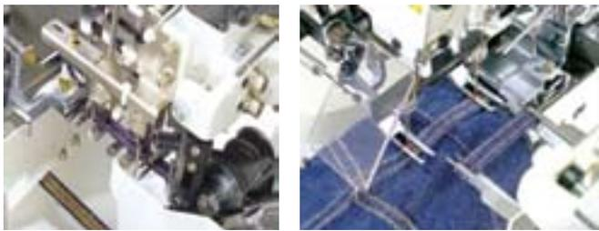
Loops being made and attached to the waistband
