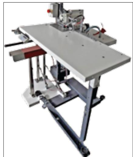
*The V800AS is the only overlock unit which can sew on the back panel with the back yoke already joined due to the patented back yoke join detector*
