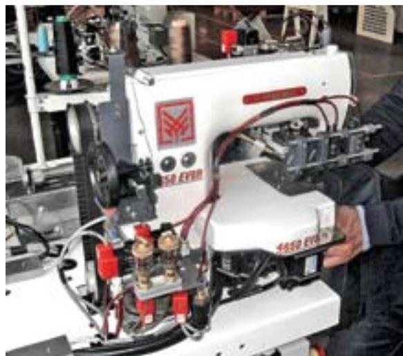
*An earlier version of the 4650EV9R automatic belt loop setter promises better efficiency and quality, now comes equipped with a completely new 7 inch coloured user-friendly touch screen panel*
